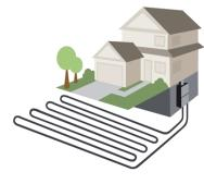
Horizontal loops require much more surface area than vertical loops and land with high moisture content is optimal as water is a better conductor of heat. Hence rural properties with large grounds which can be easily excavated are typically best suited.
