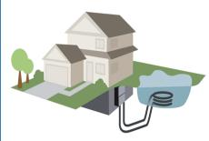
Suitable for areas with a pond or lake nearby and poor drilling & excavation conditions, where the loop can be submerged in water, rather than in the ground.
